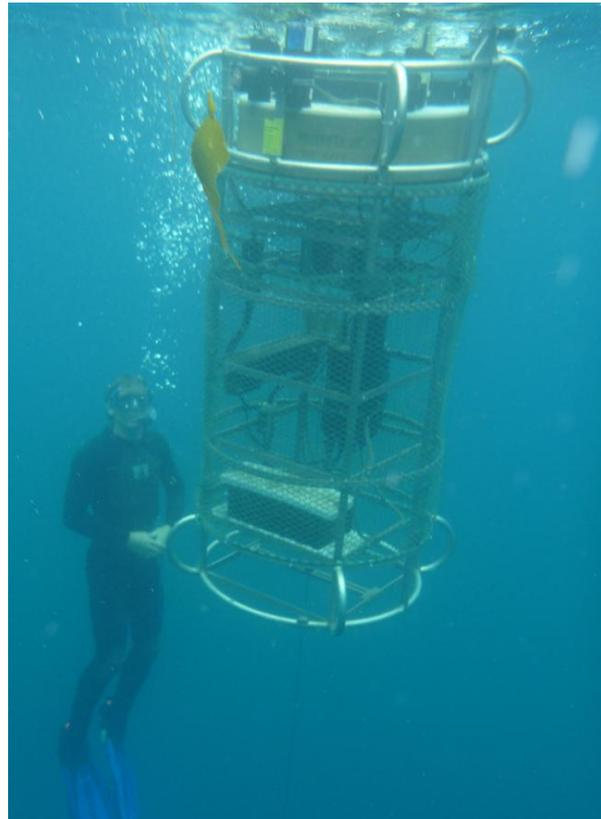
The winch is mounted in the center of the profiler, and the winch rope can be seen exiting at the center of the base of the profiler.
