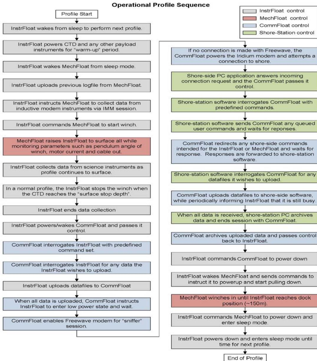
**Figure 1 GSPP Operational Profile Sequence**
