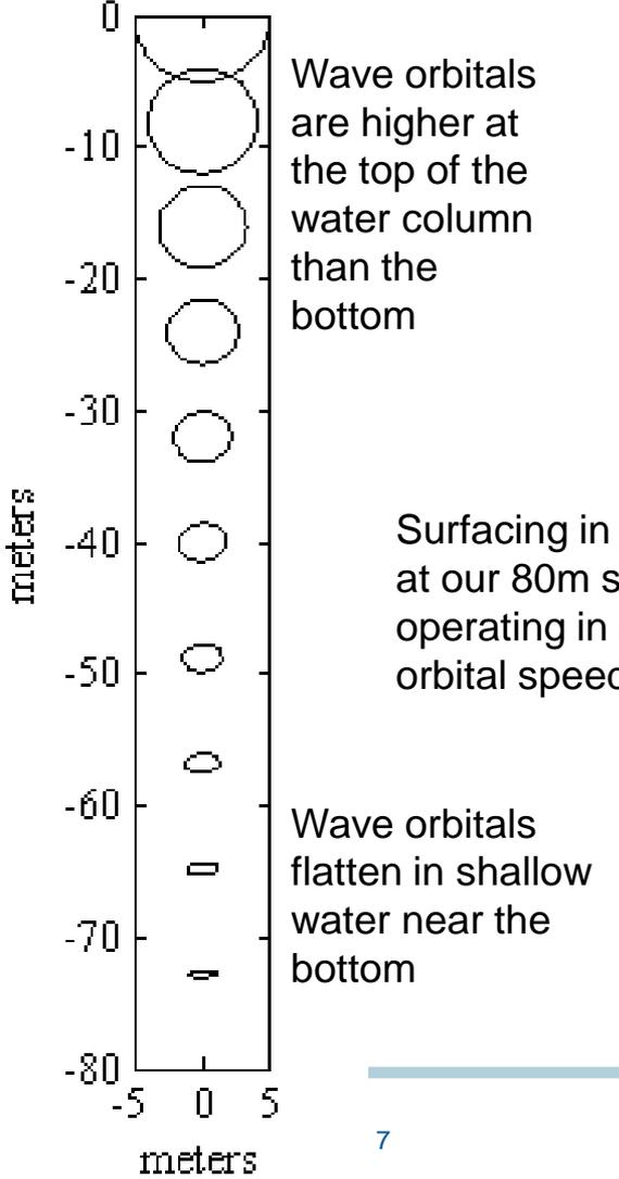
Surfacing in 3m waves at our 80m site implies operating in 80cm/s orbital speeds
