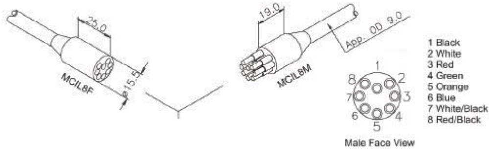
**Figure 9:** SubConn micro series pigtails are used to make waterproof connections between the riser and the buoy.
