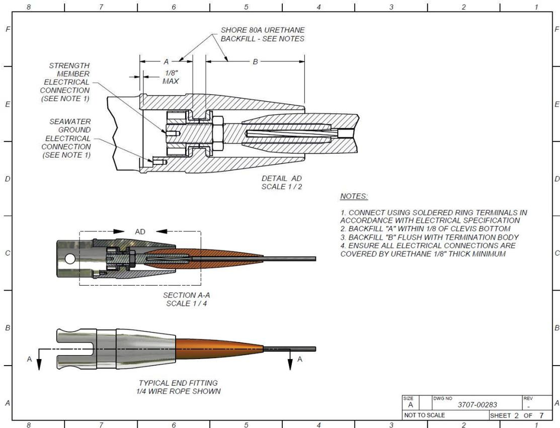
**Figure 7:** Special inductive termination isolates the strength member from the seawater ground (mechanical body).
