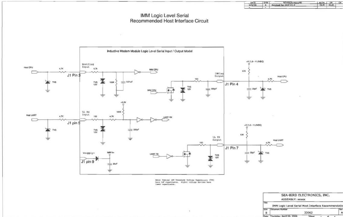
**Figure 3:** Suggested logic level Serial Host Interface
