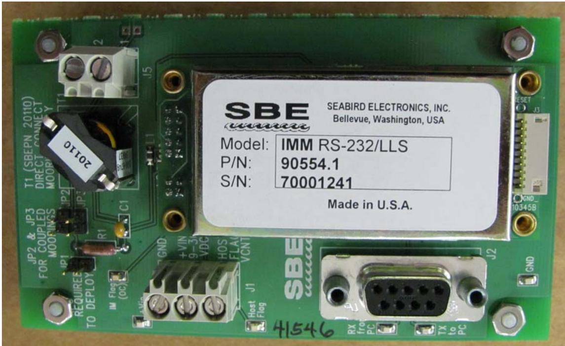
Figure 6: IMM attached to the Adapter Board.
