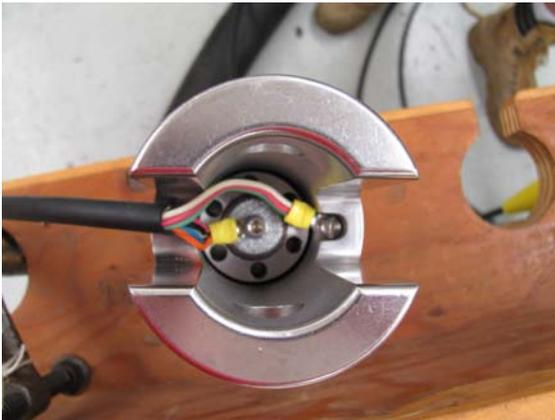
**Figure 10:** Photo showing the Inductive termination prior to potting with the underwater pigtail attached to the stud and the case or seawater ground. The stud is swaged to the strength member cable and is electrically isolated from the case using Delrin bushings.
