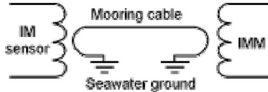
**Figure 2:** Schematic of the inductive coupling between the sensors and the IMM in the buoy (Application Note No. 92).
