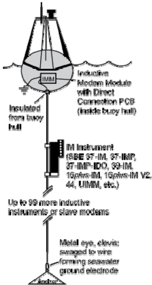
**Figure 1:** Typical inductive mooring configuration (SeaBird Application Note 92) where the application uses a direct connection to the IMM and does not use an inductive coupler.
