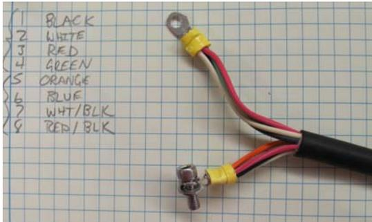
**Figure 8:** Conductors of the pigtail bundled together and crimped on to ring terminals. Four conductors each go to the strength member and the seawater ground.
